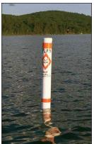
The scale shown above is the first annual results of our buoy monitoring of the water temperature at incremental depths at Pleasant Lake's deepest point(+/- 60 ft.). With sensitive data loggers spaced every two meters on a anchor line, we are able to graph over time the changes in temperature and show the
